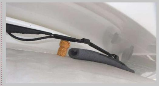
can cause it to distort. As well as using the tubing I have been taking the pressure off the blades by using a spacer between the screen and the wiper arm (making sure no windscreen washer tubes are resting on it). The ideal spacers for my boat are corks from fizzy wine.
