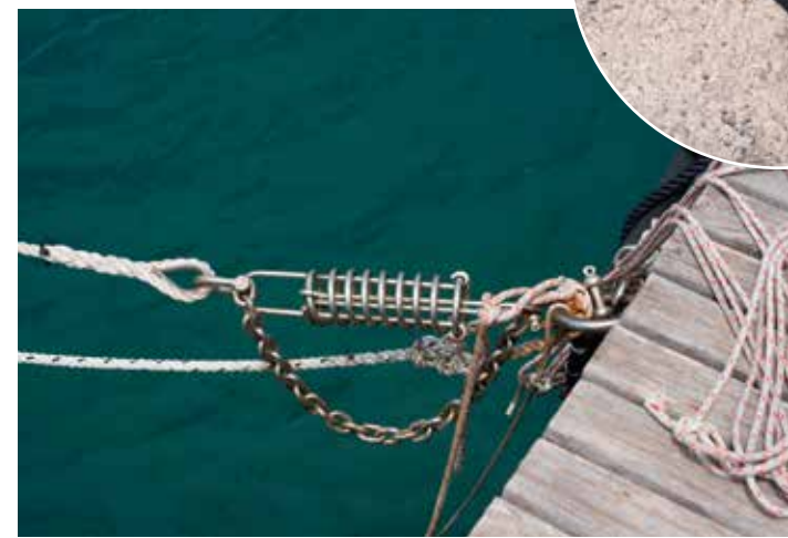
Fig. 2 Once secure this is then replaced with a heavy duty sternline fitted with chain and a snubber to reduce wear and jolting
