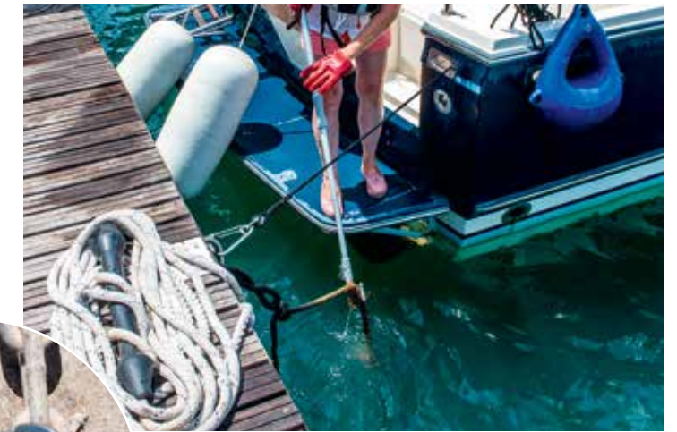
Fig. 3 Large cylindrical fenders are better at protecting the bathing platform than flat or stern fenders
