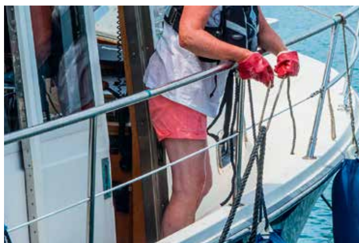
Fig. 7 Use gloves to pick up the lazy line then run it up to the bow using a piece of cord to avoid cuts and keep the dirty drips away from your decks
