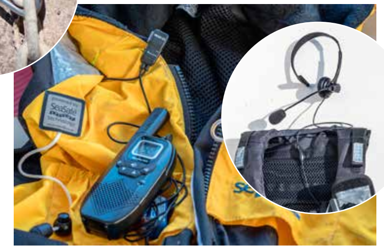
Fig. 3 Two way radios fitted with headsets make communication between skipper and crew much easier especially in windy conditions
