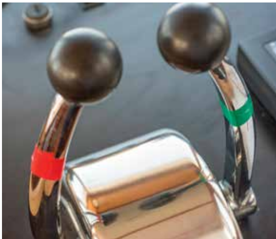
Fig. 5 Colour coded tape means the skipper can ask for a nudge ahead on red or green when directing operations
