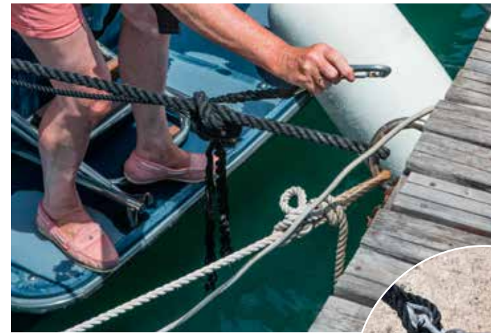
Fig. 1 A simple clip attached to a temporary stern line is much quicker and easier for crew to attach
