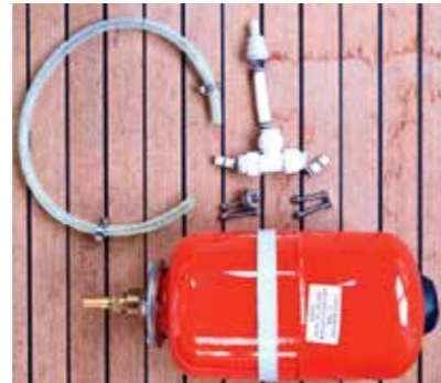
The parts needed to install the accumulator into the water system. The accumulator has a stainless steel band to hold it in place, secured with four nuts and bolts. There is also the tube spigot at the base and a valve on the top with a black cover. The push fit T-piece and spigot connector along with the connecting hose are also shown
