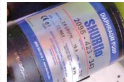
The boat has a Shurflo water pump. It's labelled as having a pressure setting of 30psi, but this is not the switch-on pressure that you need to set for the accumulator. You need to refer to the installation guide/specification sheet to find the switch-on pressure, then set the accumulator to 3- or 4psi less than that
