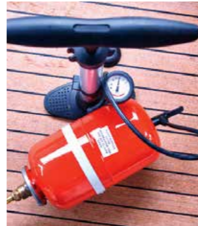
The accumulator has the same Schrader valve on the top found on cars and many bicycle tyres. Cheap and widely available bike pumps with pressure gauges fit on the valve to adjust and monitor it
