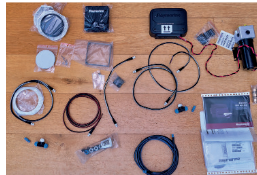
Nearly all the parts you need for installation come with the Raymarine kit, although Gilbert added some longer SeaTalkNG (StNG) cables as well as fuse holders, wire, cable ties and hydraulic hoses
