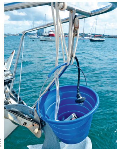
Be prepared for simple fixes such as corroded connections in navigation lights. The bucket will catch dropped components or tools
