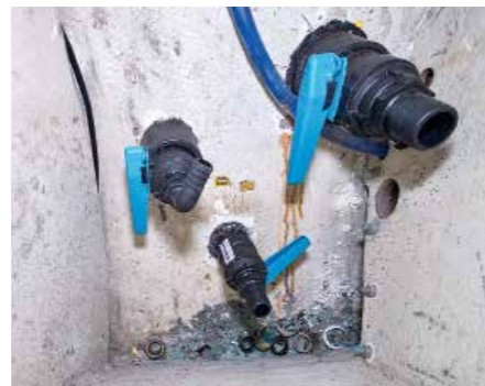
FROM LEFT Previous heads set-up; new TruDesign composite seacocks, two for the toilet one for the sink; new pipework all fitted
