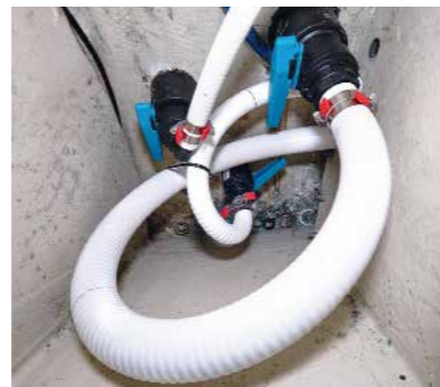
FROM LEFT Previous heads set-up; new TruDesign composite seacocks, two for the toilet one for the sink; new pipework all fitted
