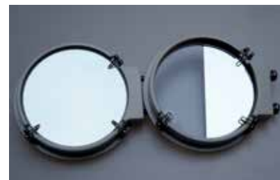
ABOVE The two main types of sextant mirror – either whole screen (left) or split screen (right) – display the view in different ways, and each has their advantages and disadvantages
