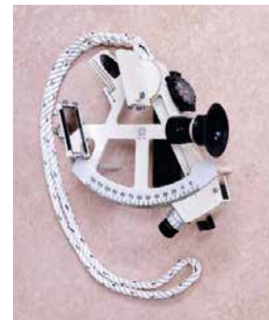
ABOVE The sextant from the boat jumble needed the mirrors professionally re-silvering, while Gilbert repaired the damaged box himself
