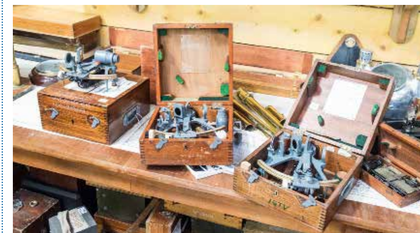
ABOVE The sextant from the boat jumble needed the mirrors professionally re-silvering, while Gilbert repaired the damaged box himself
