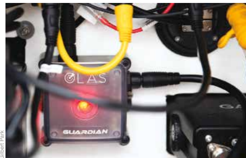
BELOW The OLAS Guardian control unit inside the console. Although it can't be seen its 85dB siren is easily heard throughout the boat
