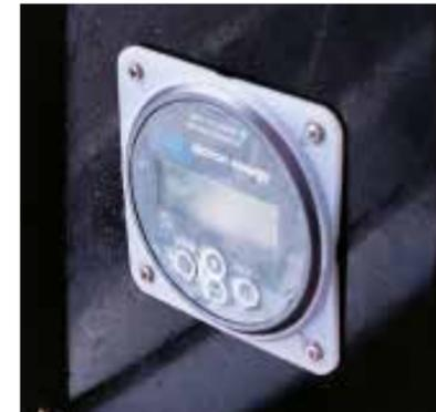
display screws onto the back and is reversible for different thicknesses of bulkhead. If access from the back is difficult then the display can be mounted using a fascia plate that it clips into. The RJ12 wire then has to be plugged into the back of the display.
