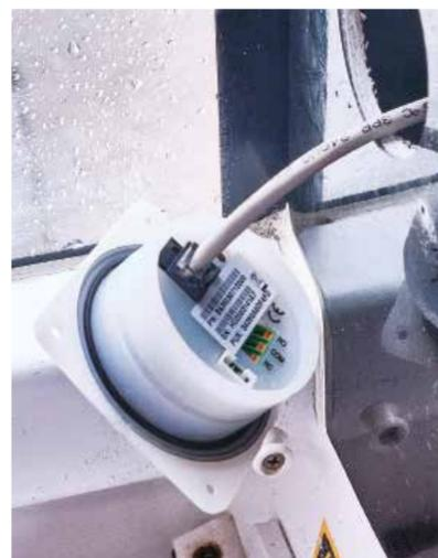
You'll need to drill a 52mm hole in a bulkhead or instrument binnacle for the display and attach the RJ 12 wire
