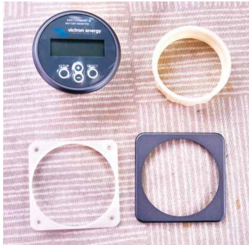
The Victron display and the options for fitting it. There is a reversible ring that screws onto the back of the display. It is reversible to allow for bulkheads of different thickness and does need access to the back of the unit. If access is difficult then the white plate can be clipped to it and screwed into place with the four small holes. It is then covered with the black trim
