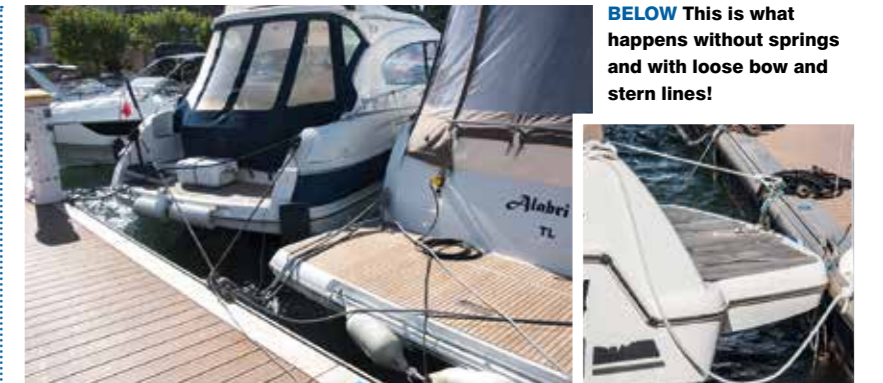
Here spring lines are stopping the boat from moving around too much. Notice that the further boat has swung around while the nearer boat hasn't. Part of the reason for that is that bow and stern lines may be tighter on the nearer boat limiting its movement. Fendering between boats remains important even when moored up
