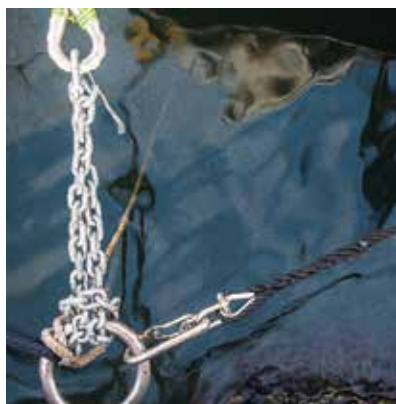
Hooks may be useful both for ease of attachment and to prevent chafing
