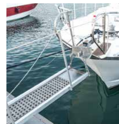
A powerboat moored bows-in. Notice the passerelle is neatly fixed to the anchor. The lazy line will be fixed to a stern cleat
