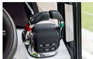
Colour coding also used to identify throttles on a twin engine boat
