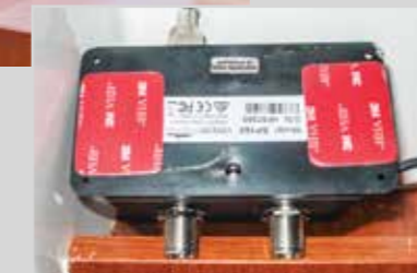
LEFT and BELOW Adhesive pads were used to simply stick some lightweight units like the AIS splitter in place
