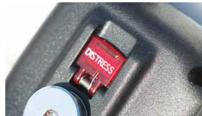
Read your DSC radio's instructions before flipping the switch to test the distress function
