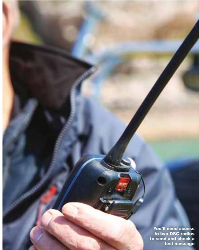
You'll need access to two DSC radios to send and check a test message
